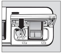
The dosage selector comes factory set to 3. It can be adjusted from 1 to 6, depending on your requirements.
